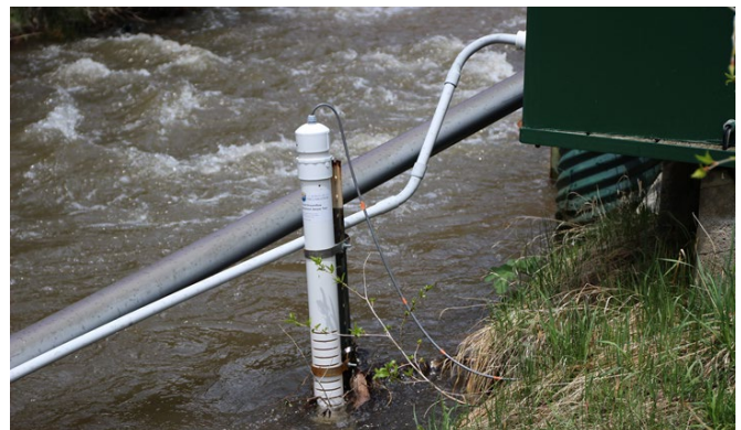
Figure 2 – eTape® sensor alongside USGS Stream Gage #06718550 – North Clear Creek near Blackhawk, CO
