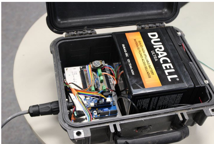
Figure 3 – Datalogger assembly using an Arduino microcontroller.
