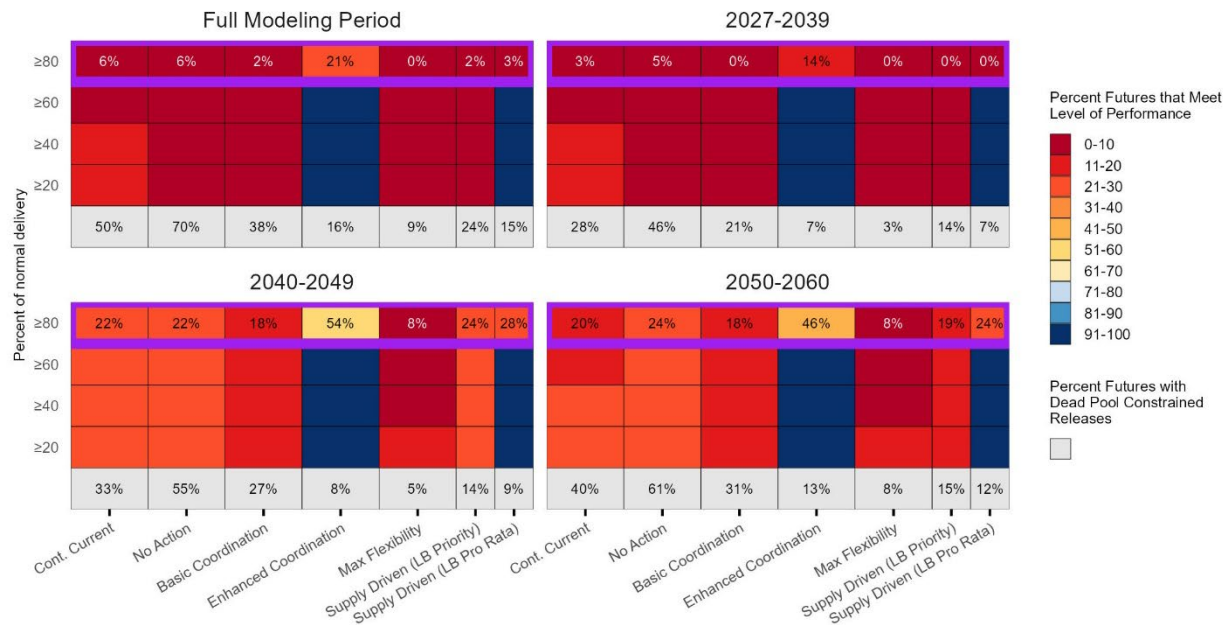
Figure TA 18-10 Arizona CAP Non-Indian Agriculture Priority: Robustness (by Subperiod). Percent of futures in which annual delivery is the percent of normal delivery specified in each row in 90% of years
