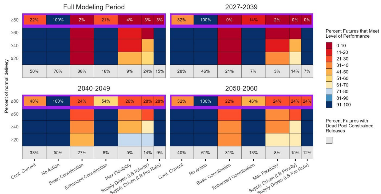
Figure TA 18-8 Arizona CAP Indian, CAP M&I, and Priority 4i: Robustness (by Subperiod). Percent of futures in which annual delivery is the percent of normal delivery specified in each row in 90% of years
