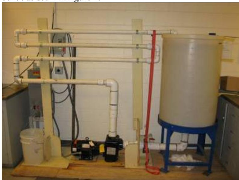
**Figure 1: High Flow Water Test set up. Samples are placed inside the PVC pipe.**
