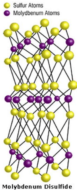
**Figure 1: Crystal Structure Molybdenum Disulfide<sup>2</sup>**
