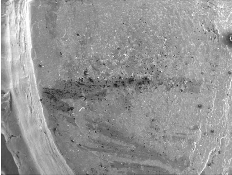
**Figure 4: Fingernail scratch visible on the end a bolt coated with WS<sub>2</sub> (35X Magnification)**
