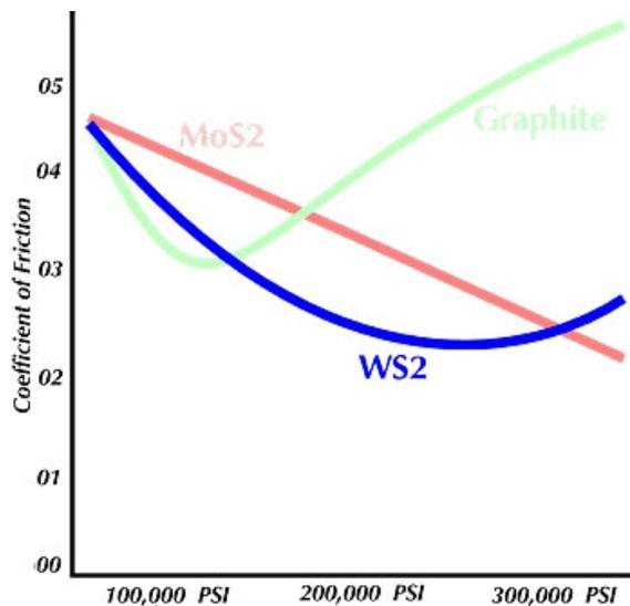
**Figure 2: Coefficient's of Friction on selected materials at various pressures.<sup>11</sup>**
