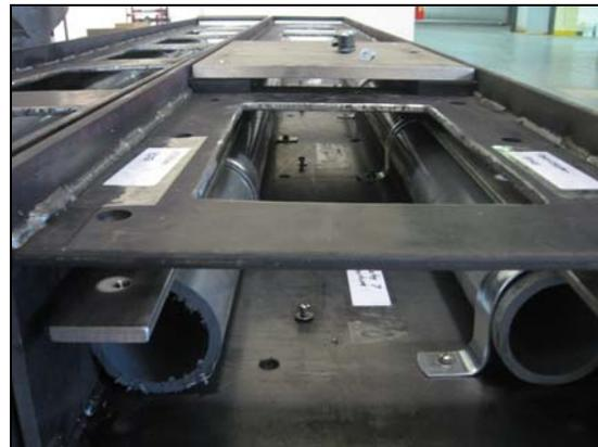
**Figure 7.** Photograph of bedload impact sensor steel plates and frames obliquely show the cross section of the assembly.
