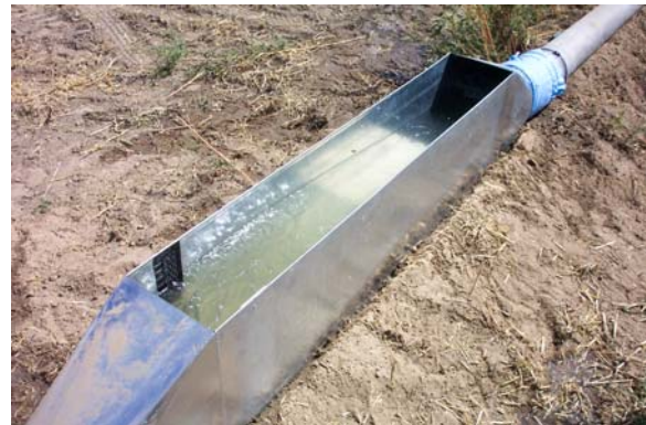
Flume installed on Pioneer Irrigation District farm turnout in southwest Nebraska as part of water measurement demonstration
