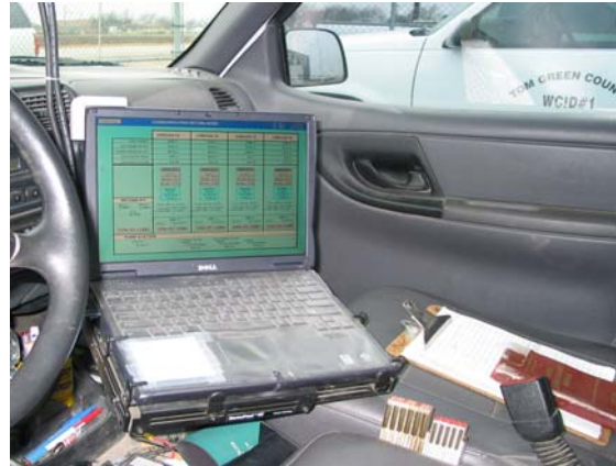
Mobile interface for monitoring and controlling canal conditions
